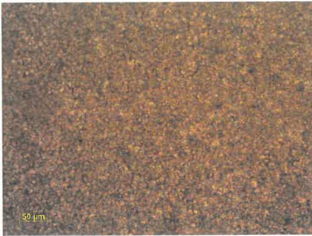
Fig 1: Photomicrograph showing microcrystalline aggregates
