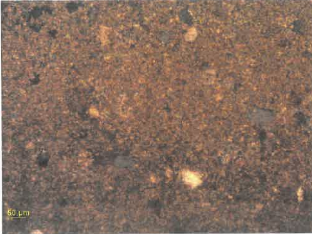
Fig 1: Photomicrograph exhibits micritic texture with presence of calcite and quartz
