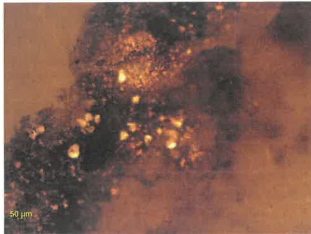
Fig 3: Photomicrograph showing calcite mineral (rhombic).
