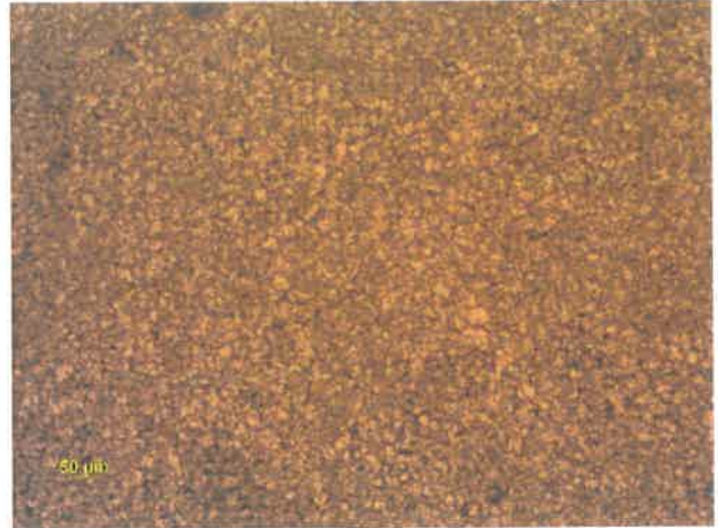
Fig 2: Photomicrograph showing presence of fine-grained calcite, dolomite.
